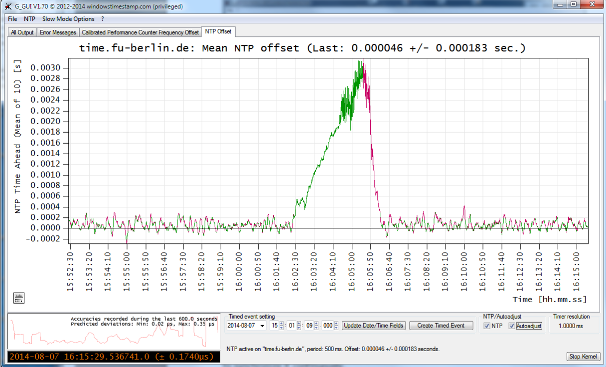
Fig. 4.4.3: Windows 7: Continuous adjustment interrupted by a three minutes drift phase.
